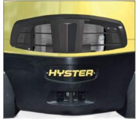
Counterweight venting improves airflow
